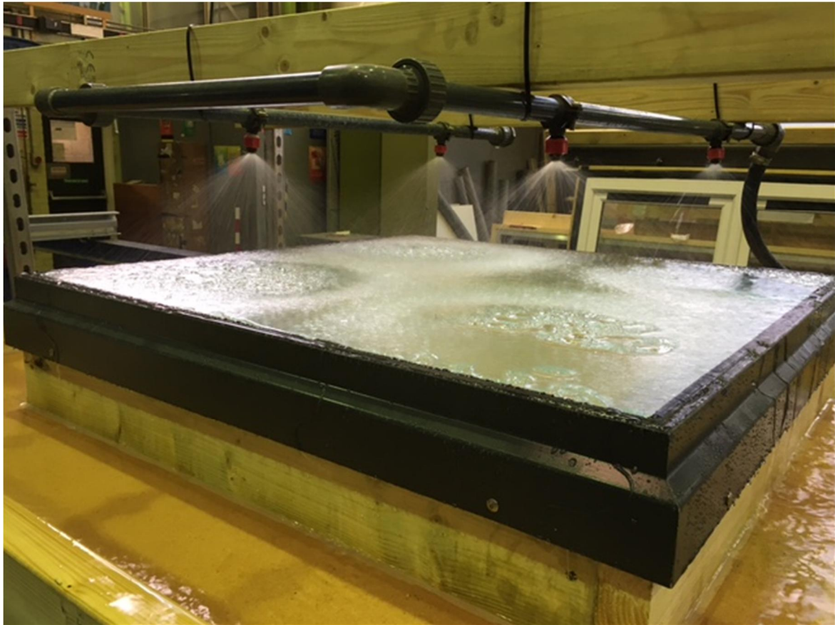
Figure A4. Roofglaze Ltd Flatglass Rooflight under watertightness test
